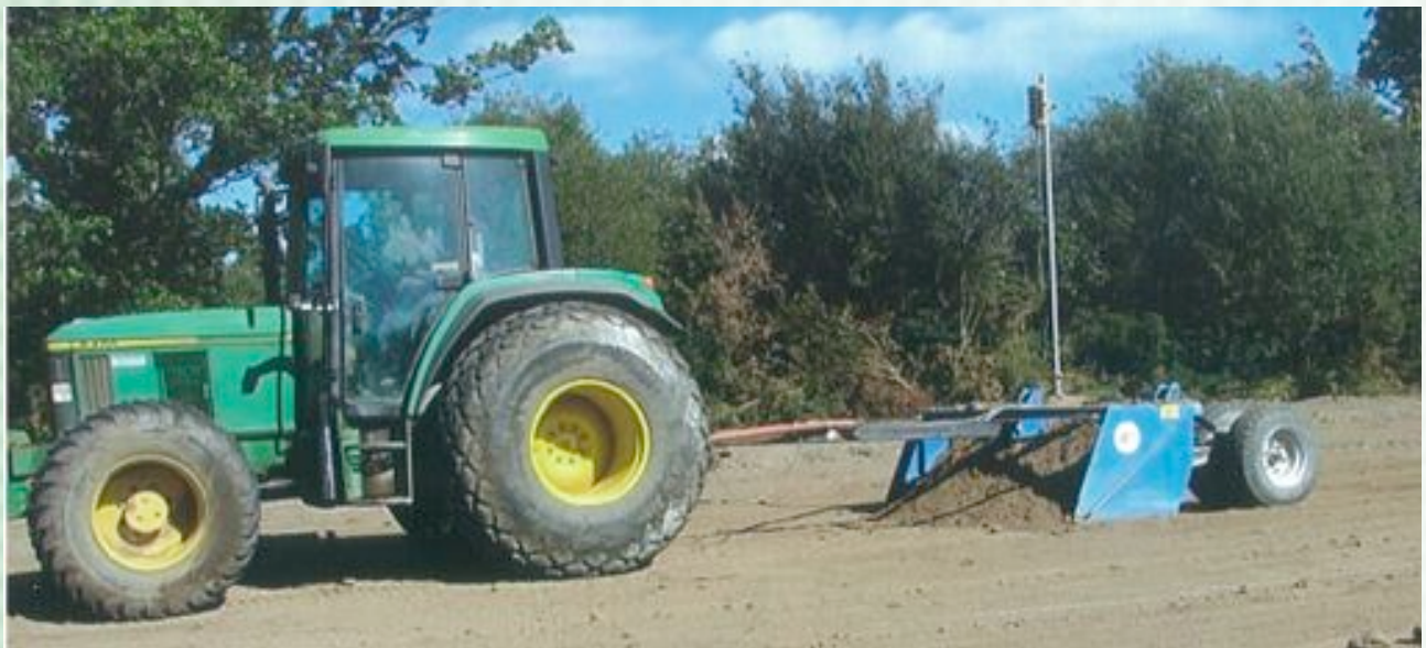
Laser Controlled Grader with Single Receiver
