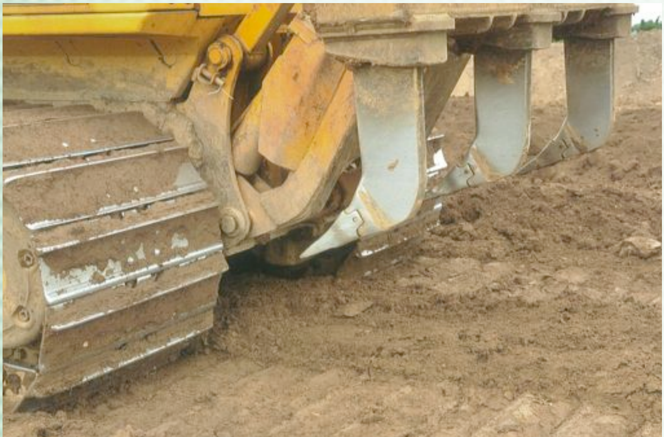
Low Ground Pressure Dozer Note Wide Pads and Ripper
