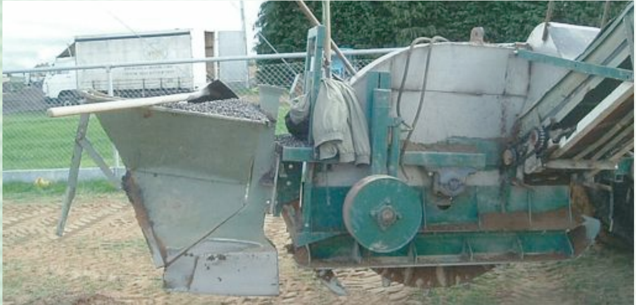
Slit Trencher with Stone Cart close to Digging Wheel
